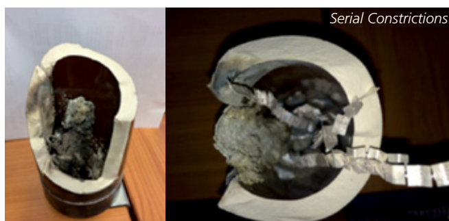
View of a failed / ruptured fuse
